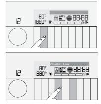
Volume level selection can be either High or Low. Menu will be opened in the level set previously. Press the 2<sup>nd</sup> auxiliary function button until the desired level appears. Desired volume level will be saved.
